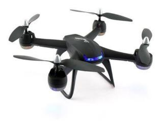
WHEN YOU HAVE ALL THE MOTORS ROTATING IN THE SAME DIRECTION (E.G. CLOCKWISE) THE DRONE BODY WILL START ROTATING IN AN ANTICLOCKWISE DIRECTION TOO.
