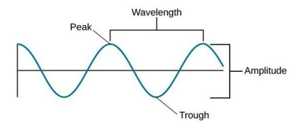
Frequency is measured in the unit **hertz (Hz),** referring to a number of cycles per second.
