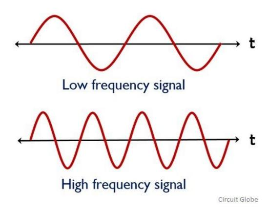
One thousand hertz is referred to as a kilohertz (KHz), 1 million hertz as a megahertz (MHz), and 1 billion hertz as a gigahertz (GHz). The range of the radio spectrum is considered to be 3 kilohertz up to 300 gigahertz.
