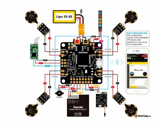
Some flight controllers include more advanced sensors such as barometer (barometric pressure sensors) and magnetometer (compass). The flight controller is also a hub for other peripherals, such as GPS, LED, and sonar sensor.
